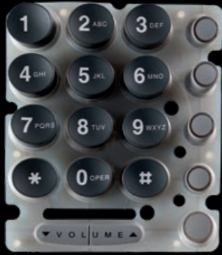
Silicone keypad with lacquered surface. Laser etched and backlit symbols.
